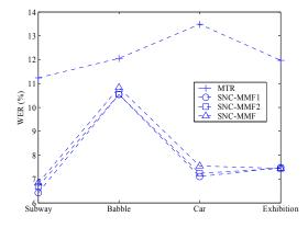
Fig. 5 Comparisons among different SNC-MMF settings and the MTR for the four known noise types in Set A
