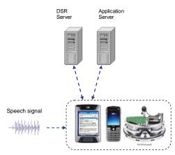
Figure 2: A distributed speech recognition (DSR) system with a recognition server and an application server.
