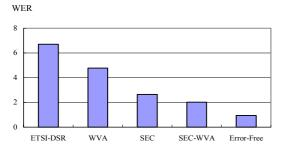
Figure 2: %WER across different methods for the GSM EP3 for Aurora 2 Test Set A.
