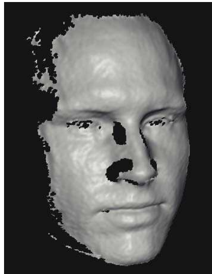
(a) Range image from structured light
