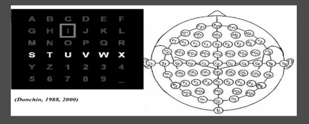
Flashing of rows/columns which contain the desired letter will elicit P300 response at vertex
